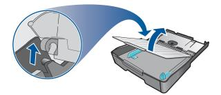
**3** To load paper between 11 inches (279 mm) and 14 inches (356 mm) long, move the latch on the tray to the right and lower the front of the tray. (You do not need to lower the front of the tray for letter-size or A4-size paper.)
